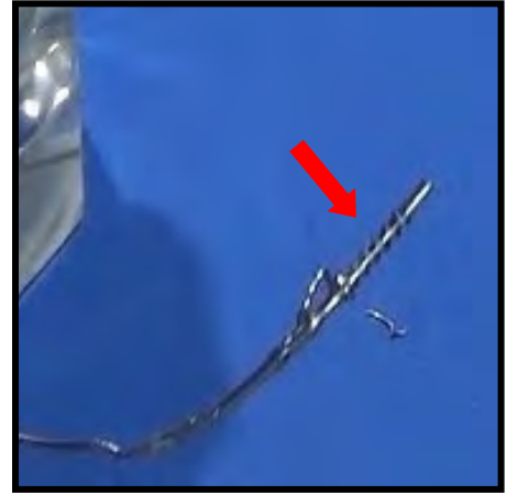
Make sure the springs are removed with the MDA.
