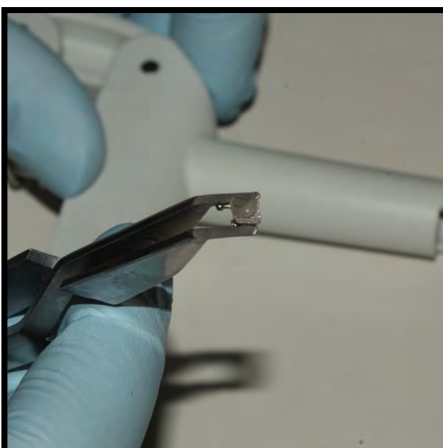
Try to get paste over the entire mesh pad.
