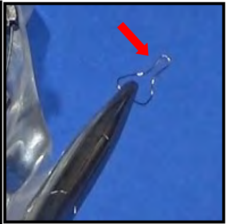
Then squeeze the end of the shorty tie together with your fingers.
