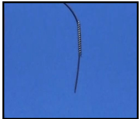
Slide the spring on the wire.
