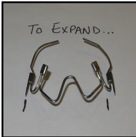
Shown is expansion from original width, with arms realigned.
